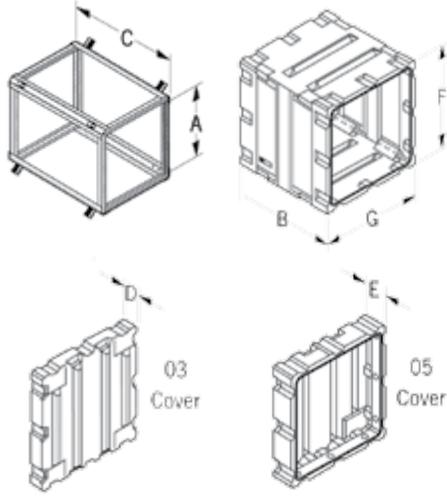
Drawing Specifications: Case Width G = 27.25 in (692 mm)
